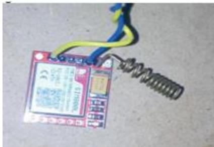
*Figure: GSM modem*
